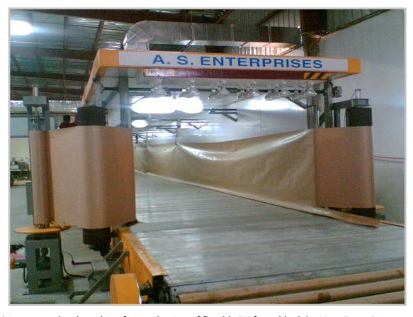
The FM200 is an entry level machine for production of flexible PU foam block by Max-Foam Process. Blocks of desired length can be cut with the help of a block cut-off machine at the end of the conveyor.
