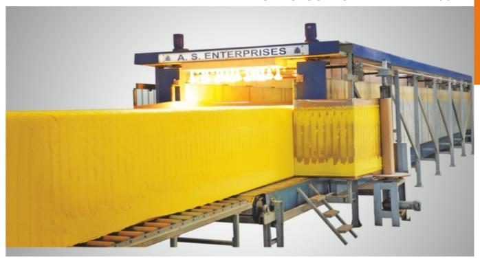
The FM400 is a high capacity machine for production of a continuous slab of flat top flexible PU foam with easy operation. Blocks of desired length can be cut with the help of a block cut-off machine at the end of the conveyor.
