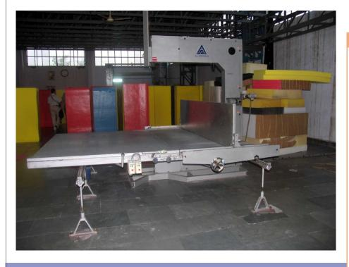
The vertical cutting machines from ASE are designed to provide a reliable means of trimming the sides of flexible PU foam blocks, and to split bigger blocks to desired sizes. These machines are also used for cutting thick sheets & sofa cushions. The cutting accuracy of these machines is +/- 2mm.
