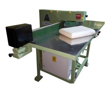
The table is adjustable in height with respect to the blade.
